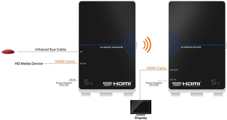
Image 7 Installation Diagram for Single Display
